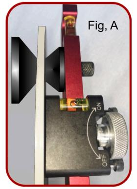
The Magnetic Aligner can be used on non-magnetic materials by using the Large set of Cones #3111-CL on the back side of flange. (Fig. A)
